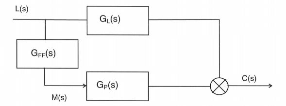
The performance of a feedforward controller depends on the accuracy of the models,  $G_p(s)$  and  $G_L(s)$ , used to design it. It will never be perfect, and, of course, it does not compensate for disturbances that are not measured and acted on by the feedforward controller. Consequently, it is common to couple a feedforward controller with a conventional feedback controller. The block diagram for this is shown on the next page.
