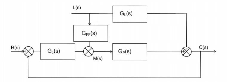
Note, in particular, that the outputs of the two controllers are simply added together.
