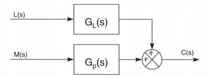
The diagram shows both the manipulated input, M(s), and the disturbance input, L(s), influencing the measured variable, C(s). This is shown in the form of a linear model, which will typically be an approximation to the actual behavior, i.e., a transfer function fitted to response test data.
