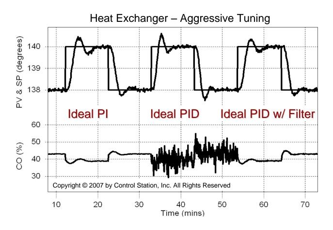
• IMC tuned ideal algorithm: PI vs PID vs PID w/ CO Filter
