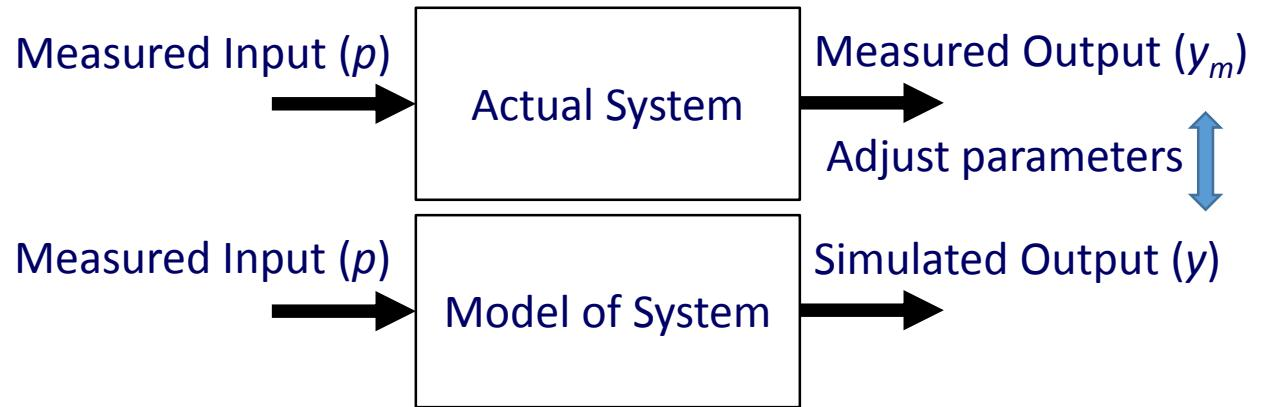
$$\begin{aligned} & \text{minimize} && \|y_m - y\|_n \\ & \text{subject to} && 0 = f\left(\frac{dx}{dt}, x, y, p\right) \\ & && 0 \leq g\left(\frac{dx}{dt}, x, y, p\right) \end{aligned}$$
