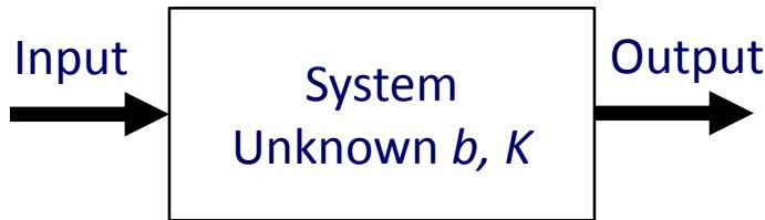
$$\begin{aligned} & \text{minimize}_{K,b} && (v_m - v)^2 \\ & \text{s.t.} && \frac{m}{b} \frac{dv}{dt} = -v + K p \\ & && 0 \leq b \leq 100 \end{aligned}$$
