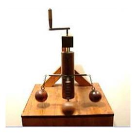
We propose a slight variation of da Vinci's design, replacing the chains with springs. This increases the energy that can be stored in a flywheel as some of the energy goes into stretching the springs. We will try to maximize the additional energy per unit mass that can be obtained from this design. Some simplifying assumptions that we make are:
