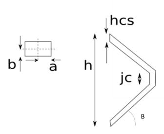
For the objectives we will define size as the sum of the height and the outer diameter. We want to set an upper limit on the force of 3 lbs to cause a deflection  $\delta$  of 0.1 inches. The spring must also not be allowed to clash (reach its solid height).
