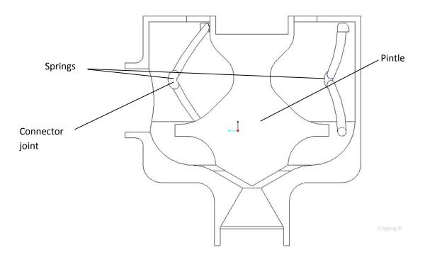
We wish to optimize the helical spring to achieve the smallest design while minimizing the amount of axial force necessary to actuate the valve. The stress in the spring legs should be below the yield stress and the design must conform to manufacturing constraints.
