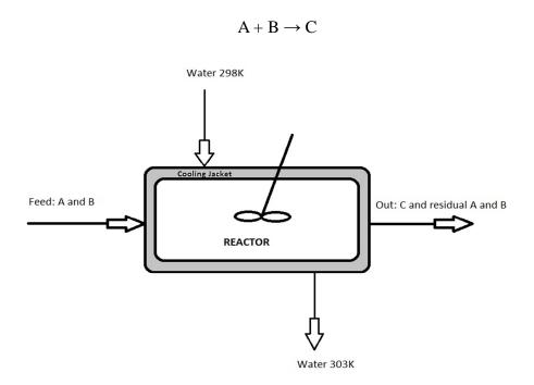
A continuous-stirred tank reactor (CSTR) has a flow of A and B going into it to form C. The reactor is kept at a constant temperature by a cooling jacket surrounding the reactor. The profitability of this design is based on how pure the C is coming from the reactor. To maximize profit you need to provide the optimal reactor volume, reactor temperature, mass flow of water through the cooling jacket, and feed rate of compounds A and B.
