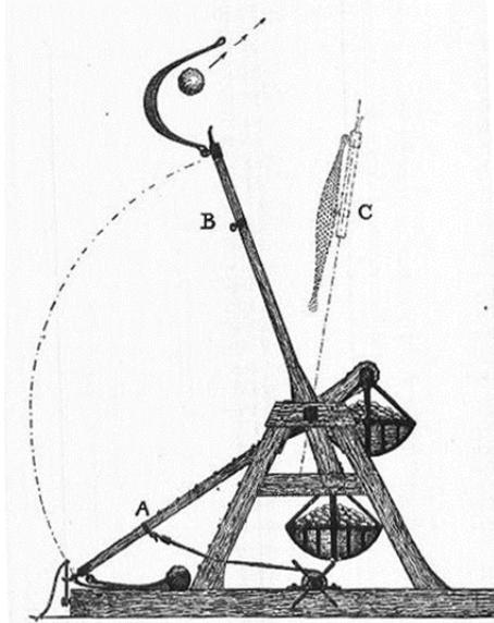
Trebuchets are designed with many trade-offs in mind. The longer the arm, the farther the projectile will go. But then the base has to be expanded and the device quickly becomes very expensive. Use APM to maximize the range of a given geometry using time of release as the variable. Next, choose several geometries and find the configuration that gives the maximum range per dollar.
