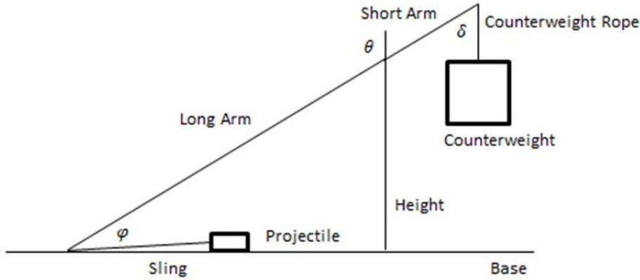
The counterweight has a mass of 100 lb, the projectile has a mass of 1 lb, and the mass of the arms (long and short together) will be 5 lb no matter what their length is optimized to be. The length of the short arm is 1 ft (L1), the length of the long arm is 7.5 ft (L2), the length of the sling is 3 ft (L3), the length of the counterweight rope is 1 ft (L4) and the height of the pivot is 5 ft (L5). The initial condition of the angles can be calculated using the following equations:
